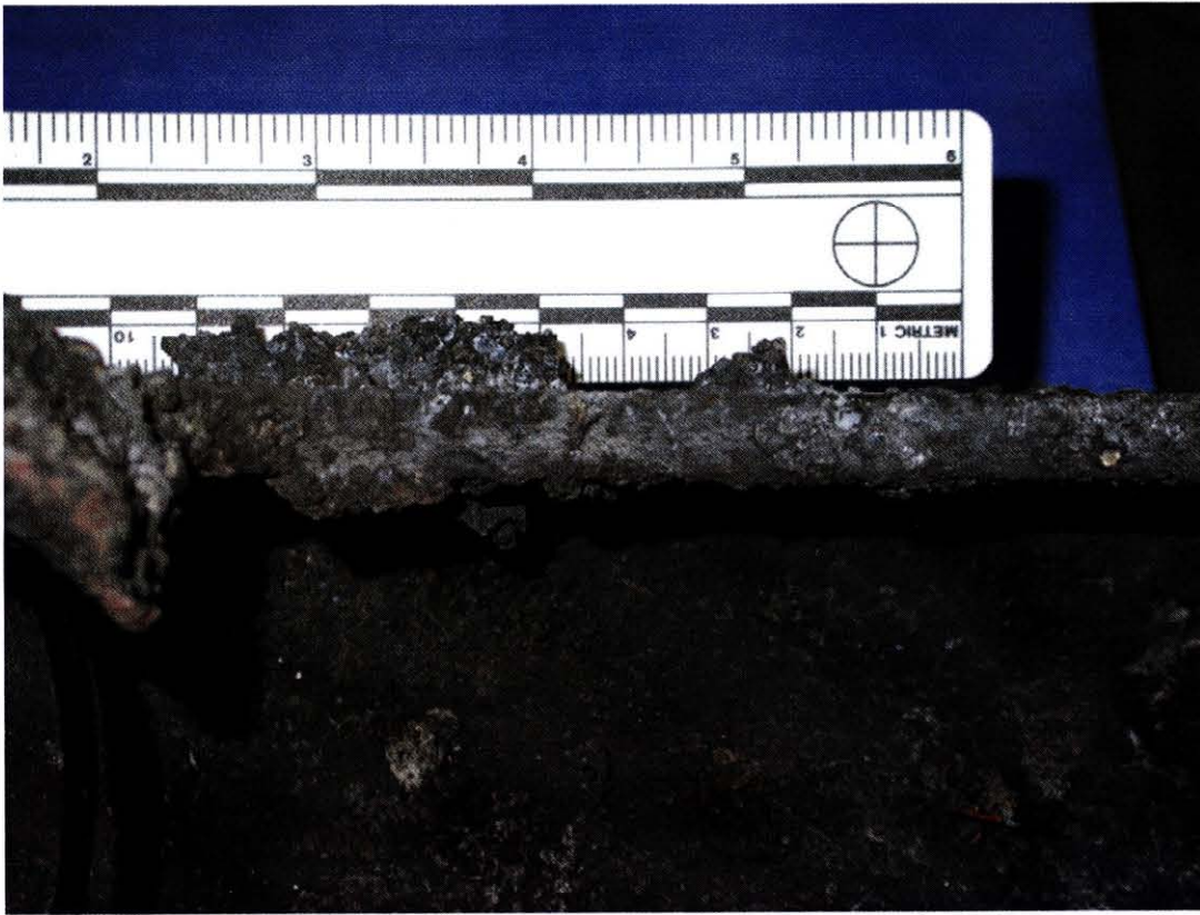
Figure 32: Slag Deposits on Upper Edge of Panel 8 on the RCC Side of the Vent.
