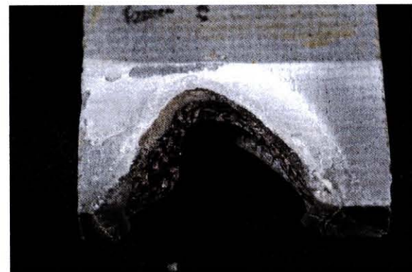
Figure 44 (c): Close Up, Post-test Photograph Showing Knife-edges in the RCC Closeout.
