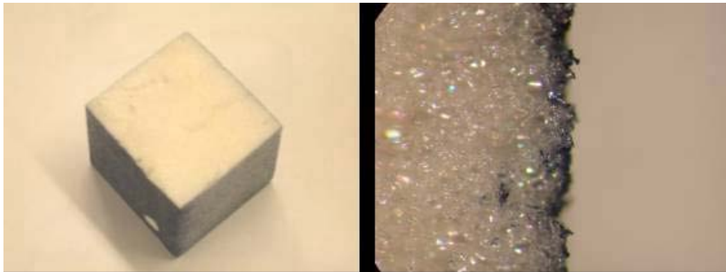
Figure 2. (a) Shows blue dye decorating the surface of a BX-250 foam cube that was submerged 26.5 hours then sectioned, revealing the interior. (b) Shows a magnified image at the sectioned surface.
