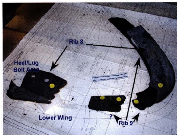
Figure 28: RCC Panel 8/9 Ribs (Outboard View).
