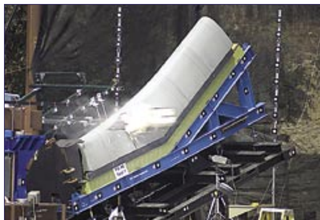
Figure 3.8-5. A typical foam strike leaves impact streaks, and the foam projectile breaks into shards and larger pieces. Here the foam is striking Panel 6 on a fiberglass test article.
